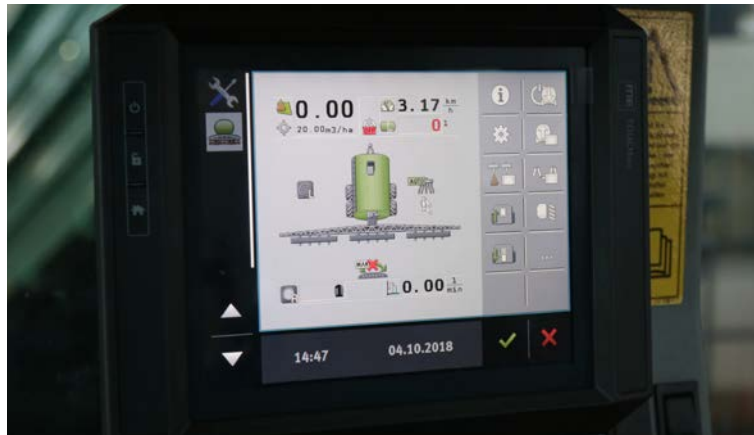
Bedienterminal ISOBUS TOUCH 800
